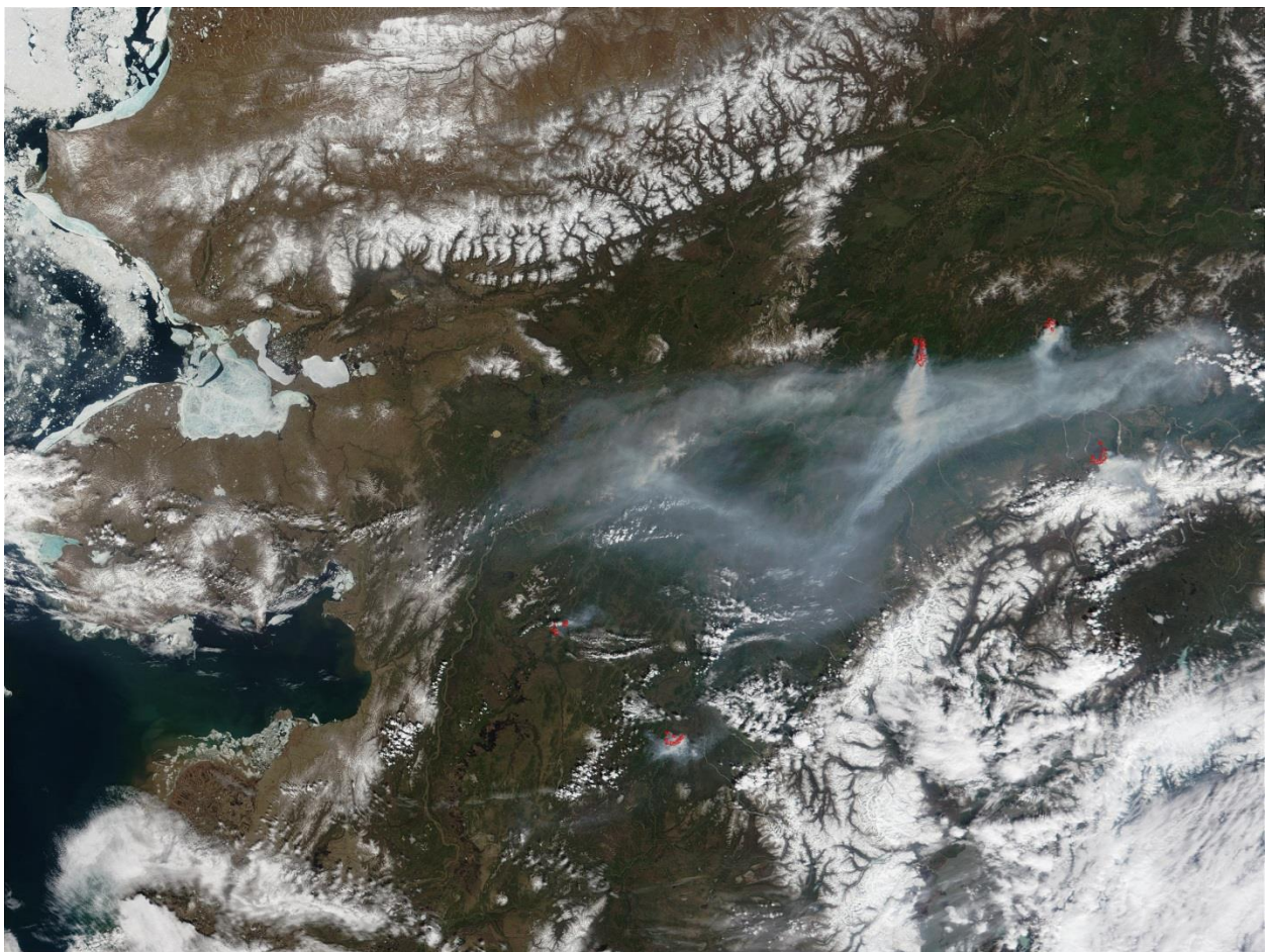
Figure X. MODIS scene of western Alaska USA, collected on 26 May 2002. The red polygons represent hot-spot algorithm-detected regions. Associated smoke plumes can be seen, as well as snow-covered regions, and areas of sea ice.
