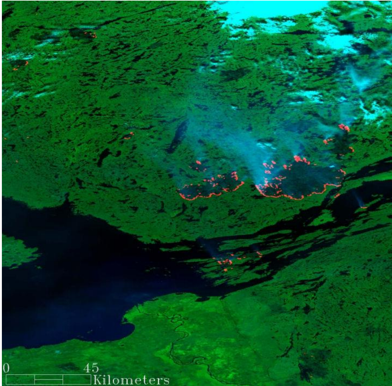
Figure x. VIIRS I-Band (375m spatial resolution) fire detection for a wildfire at Great Slave Lake, NW Territories, Canada collected on 14 July 2014. Note the improved spatial detail of the I-band data.
