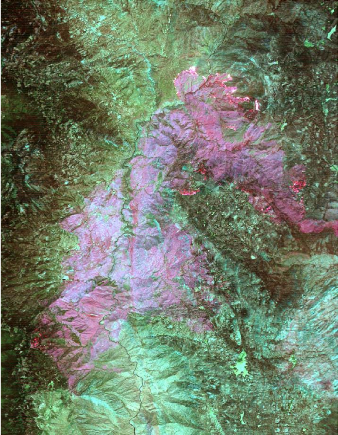
Figure x. eMAS data collected over the McNally Fire, California on 6 August 2002 The burned area can be seen in light red hues, while the active fire front is seen in the upper right edges of the burned area as yellow and white areas. This composite is composed of the following spectral channels: 21, 10 and channel 2.
